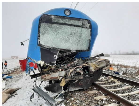
Photograph 2 - Consequences of the occurrence - the damaged EMU EN57AL-1527 (source: own material of PKBWK)
