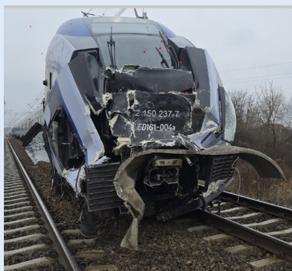
Photograph 18 - Consequences of the occurrence - the damaged ED161-004a cab (source: materials of the railway commission)
