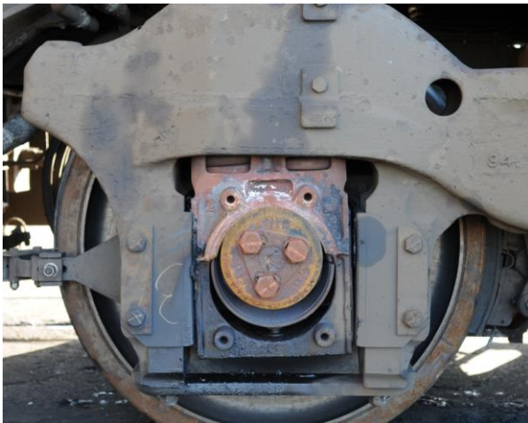
Figure 7 – Failed bearing on locomotive 233
