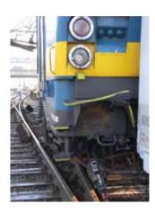
On 9 March at 04.53, the last carriage of the passenger train leaving Mons in the direction of Saint-Ghislain derailed on points 43B in the 'grill' just outside Mons, damaging several sets of points.
