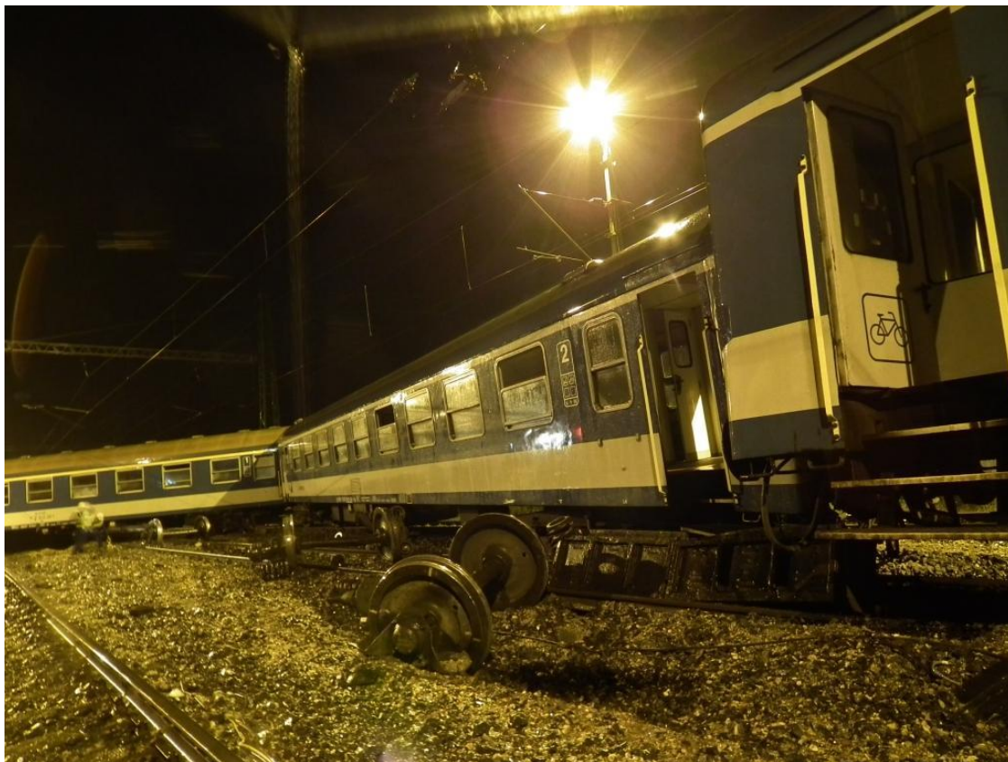
The derailed carriages of train No. 9021 at Ostffyasszonyfa station (Photo's courtesy of the Hungarian NIB)
