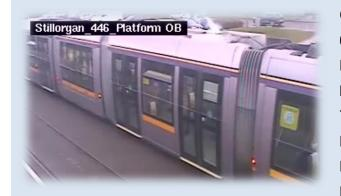
On 2<sup>nd</sup> November 2020 the 14:31 hrs Luas Service 65 (operated by Tram 5010) from Brides Glen to Broombridge served Stillorgan inbound platform before moving forward to Signal B11. The driver of Tram 5010 (Driver 5010) noticed the Main Circuit Breaker (MCB) had opened in the driving cab (the MCB opened due to its failure to detect 750 volts (V) Direct Current (DC) from the Overhead Contact
