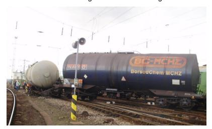
investigation The established that the spindle the of wagon had already been faulty, had fallen apart and the bearing box had fallen off the wagon right before the occurrence, which resulted in the derailment the of wagon.
