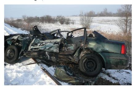
The IC examined the structure and operation of the level crossing and established that the warning lights were flashing red lights toward the road at the time of the accident. The train was not exceeding the speed limit.
