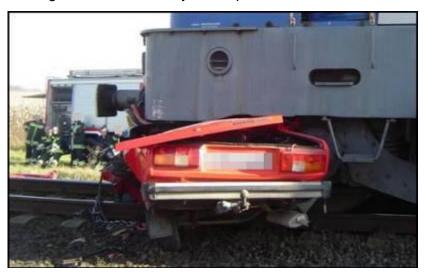
The IC considers that the driver of the car was not approaching the level crossing with due foresight and entered it ignoring the "Stop" indication of the warning lights closed and the position of the halfbarriers. He could not exit the level crossing before the train arrived and this resulted in
