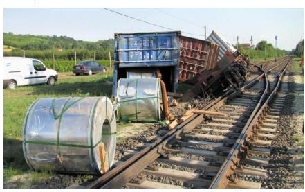
the last track section before points no. 4. The engine driver. realizing the occurrence of accident. the used the emergency brake. this resulting in the rupture of the screw coupling of wagon no. 83 35 549 6518-2 and the split of the train. The IC
