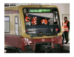
On Monday, 20 November 2006, a collision occurred at Südkreuz station in Berlin between a suburban passenger train and a Sperry SRS 200 rail test car. The suburban train was following the test car at a distance. Although its emergency braking system was activated, the suburban train did not come to a halt soon enough to avoid the test car, which had stopped in the station.
