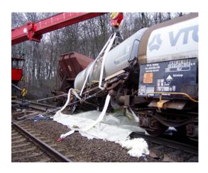
Goods train 51245 collided with goods train 50216, the latter being stationary at the home signal, which was displaying a stop aspect, at Kalk Nord goods station, Cologne. The collision caused the derailment of eleven wagons belonging to train 51245, some of which were tipped at an angle.
