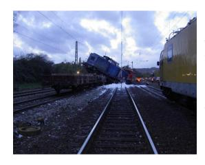
At Obervellmar station, goods train 44983 collided with a shunting train emerging onto the running line from a sorting siding. Both power units and the first wagon of each train were derailed.
