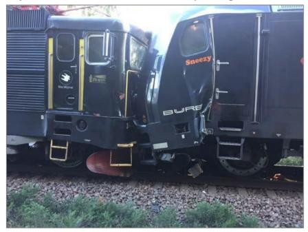
On 30 September 2016, a freight train was stationary in an upturn between Deje and Molkom on the Kil – Daglösen single-track stretch. An auxiliary vehicle, consisting of two Rc3 locomotives, was sent out to help the stationary train. However, the auxiliary vehicle collided with the train, one of the drivers was injured and the vehicles suffered extensive damage.
