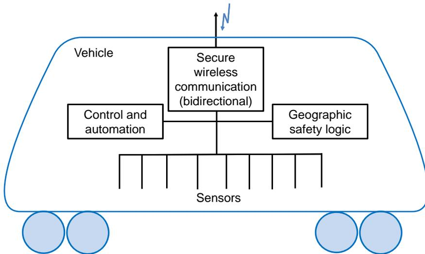
Figure 6 –Representative architecture of the on-board system with Command and Control 4.0.
