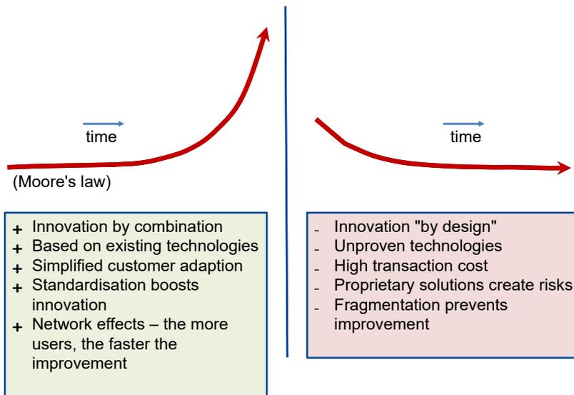
Figure 1 – Combinatorial innovation (left) leading to improvements on an exponential scale, in comparison with the approach often followed in rail (right). Innovation “by design” also means that use of the so-called Vee Model, often called for in safety assessments (as for example in CENELEC EN 50128), is required.
