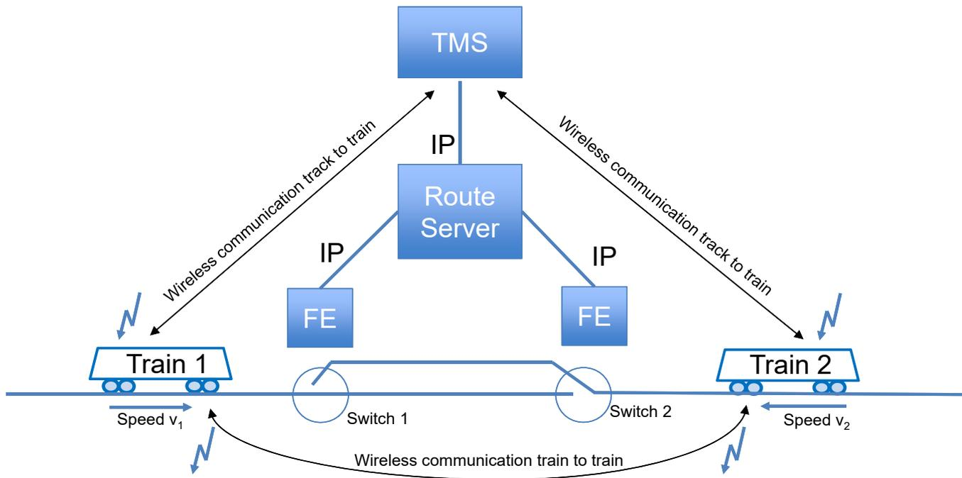
Figure 5 – Architecture of a future Command and Control 4.0 system. Smart wayside objects (field elements, FE) have open interfaces and powerful degraded modes. On the train, clearly only one interface is necessary, the communication interface between the rail vehicle and the external world.
