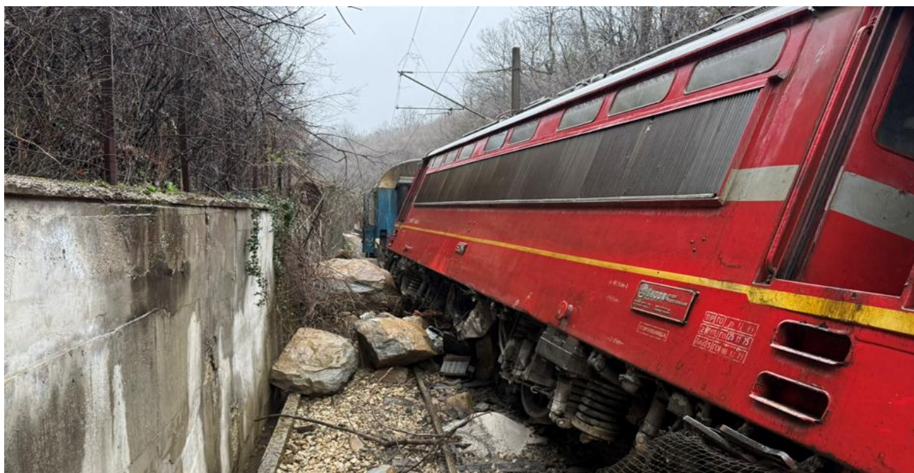
Fig. 1.3. Locomotive No. 91520044191-2 of FT No. 4631, derailed with all wheelsets
