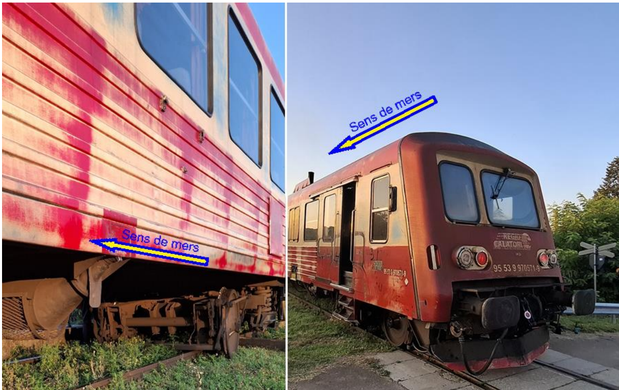
Photo no. 1: the AMX 571 diesel multiple unit in a derailed state
