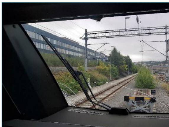
Figur 10: Sprekk i frontruten. Foto: Stadler Service Norway AS
