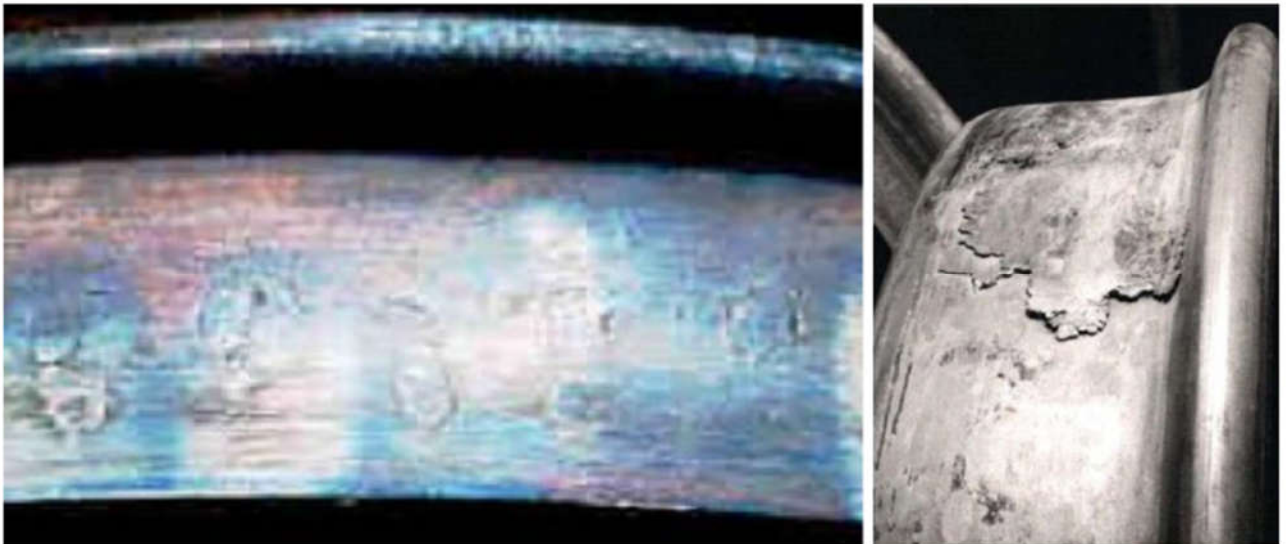
Figure 9: Signs of thermal overload of the wheel - discolouration of the tread and metal build-up on the tread
