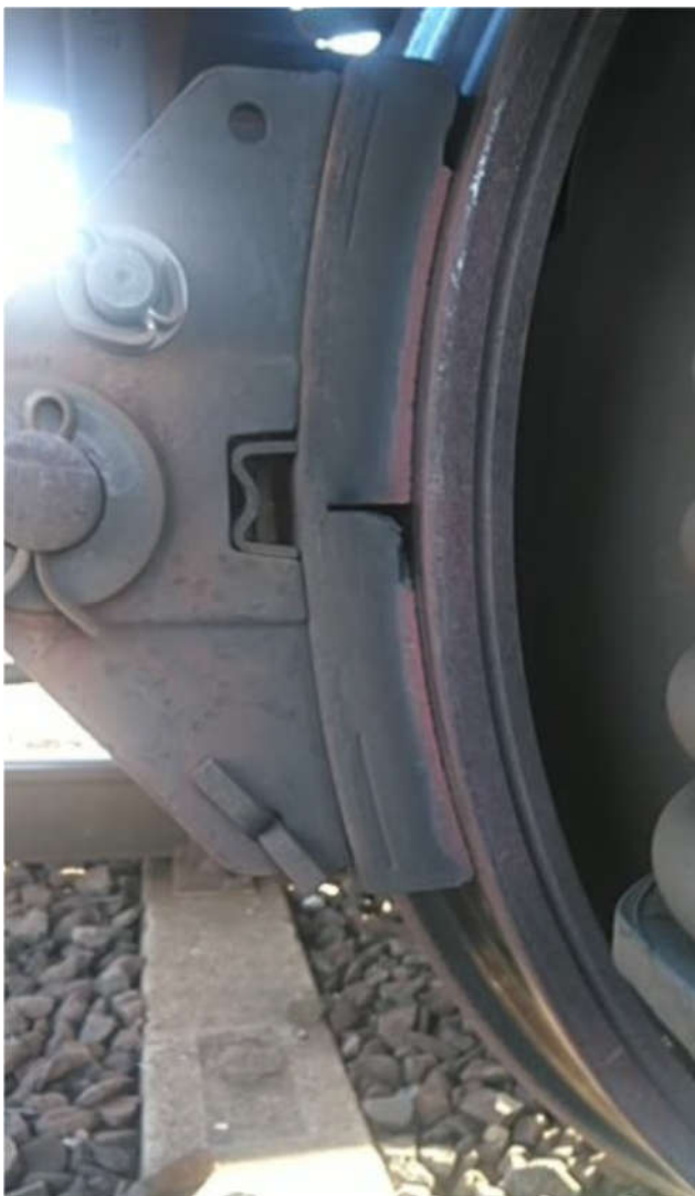
Figure 2: Organic brake blocks: 'Red layer' in the rubbing surface, up to 10mm thick [UIC Leaflet e541-4, 3. Edition]
