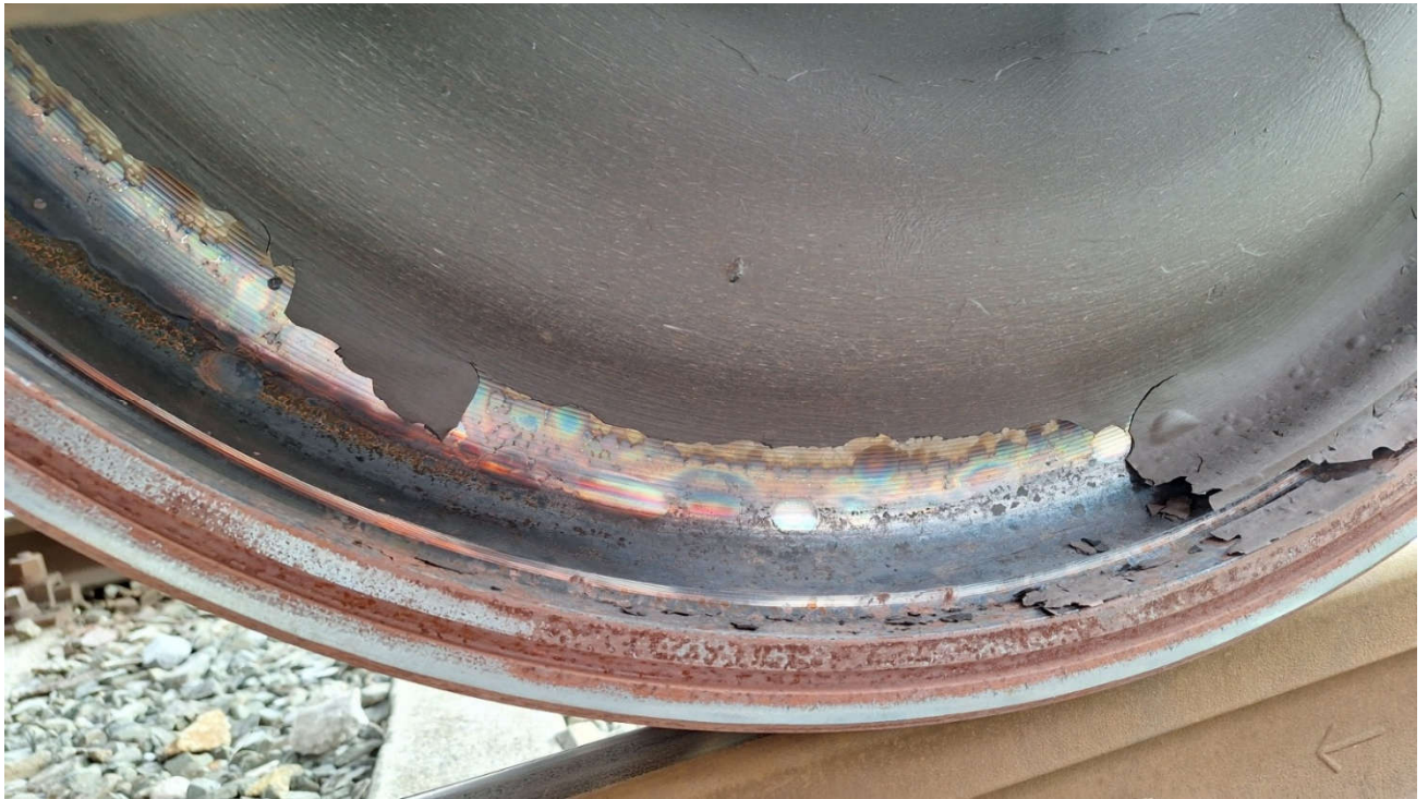
Figure 8: Signs of thermal overload of the wheel – burnt paint
