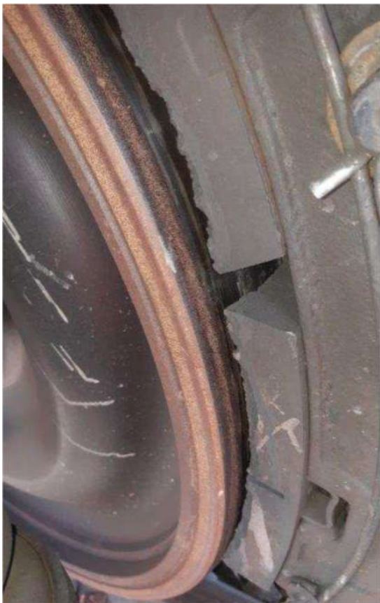
Figure 4: All type of brake blocks: Crumbling of the rubbing surface, friction carbon deposits high, up to 10mm thick [UIC Leaflet e541-4, 3. Edition]
