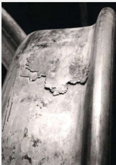
Metal build up on the tread
