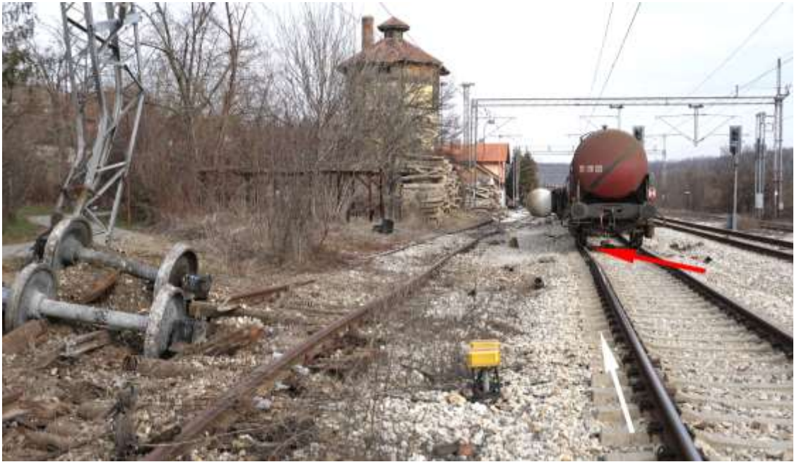
Figure 4.2.10.5: Position of detached wheelsets and overturned tank wagon
