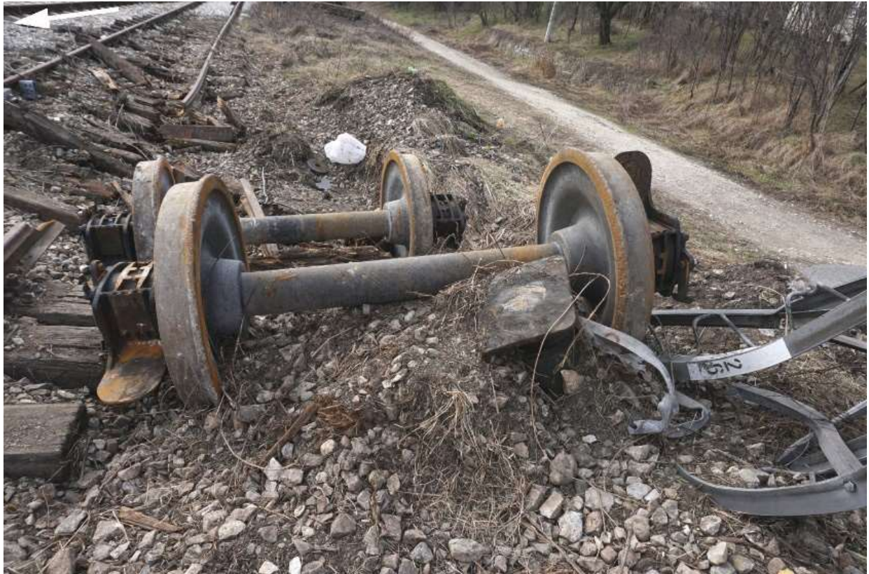
Figure 4.2.10.4: Detached wheelsets and buffer of the eleventh wagon
