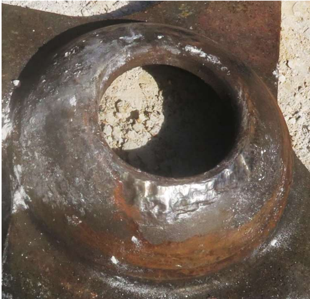
Figure 4.2.13.4: Upper center bowl of the respective bogie
