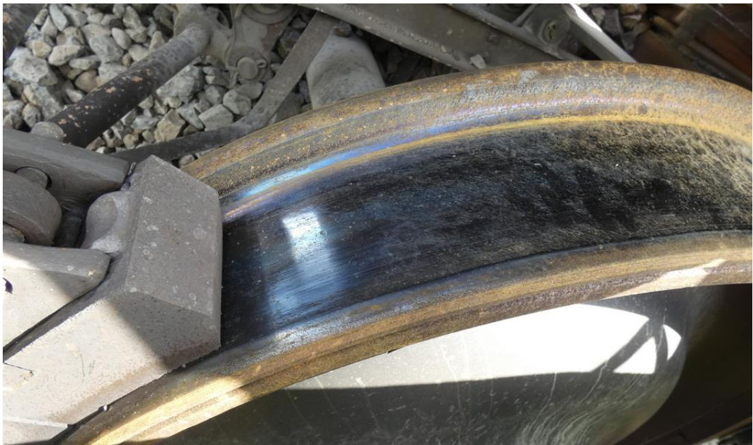
Figure 5: Discoloured wheel in the second bogie of the wagon with reg. No. 470-4 (contrary to what the picture suggests, the tread is not damaged, there is no external pseudo-marking on the wheel)
