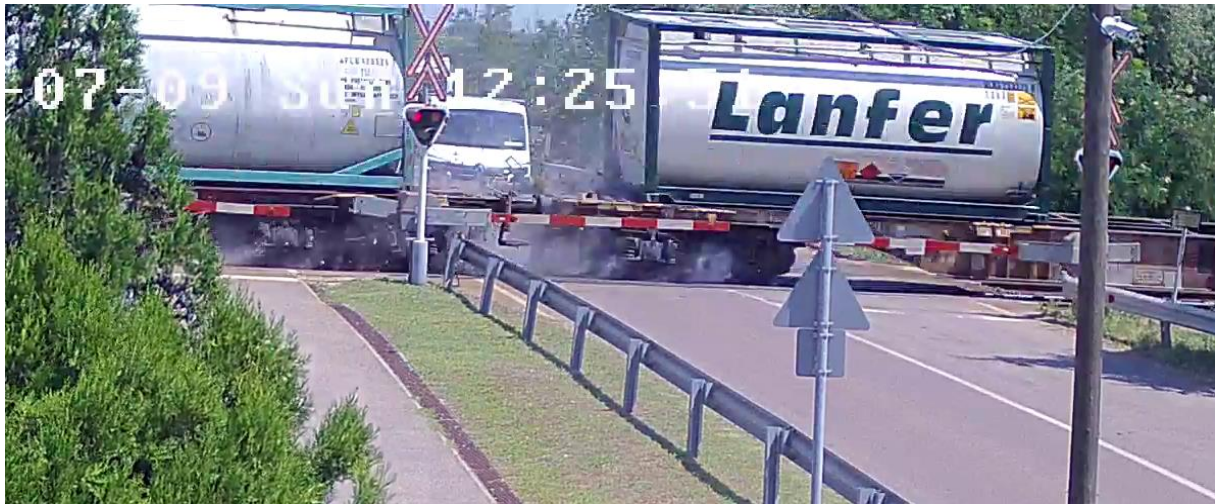
Figure 3: Part of a frame of a surveillance camera image, showing the derailed bogie reach the level crossing
