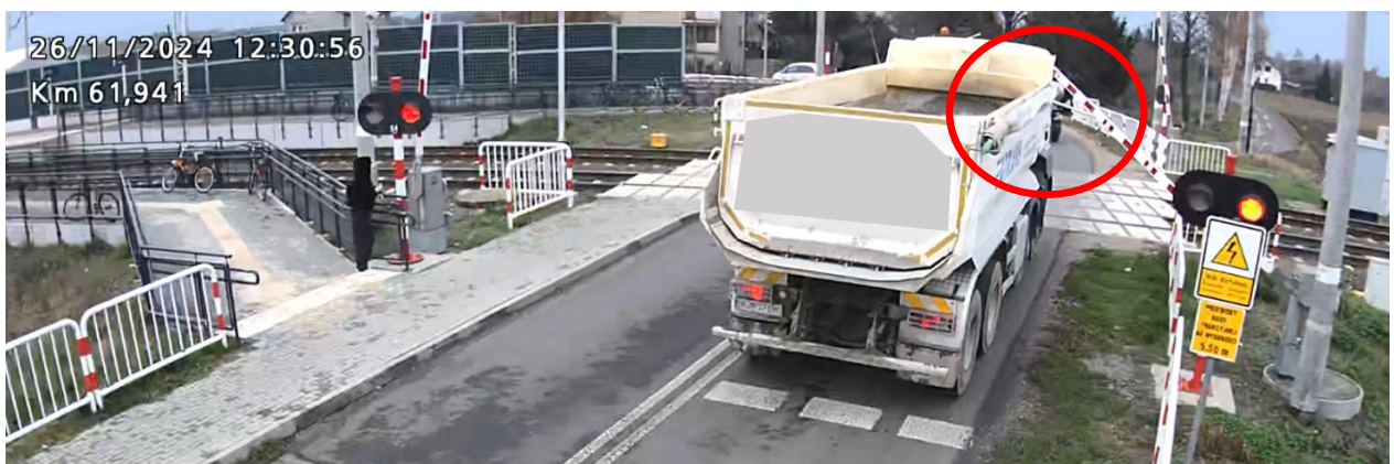
Photograph 8 – A view from the camera from the side of the N2 drive showing the lorry entering the crossing and the barrier being bent (source: PKP PLK S.A.).
