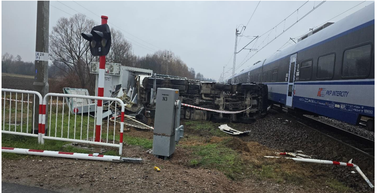
Photograph 1 – The consequences of the occurrence in the area of the crossing – damage to the infrastructure and equipment prohibiting entry to the crossing (photo by the railway commission)
