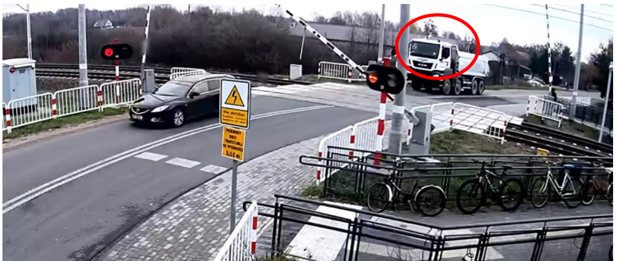
Photograph 7 – A view from the camera from the side of the N1 drive showing the lorry entering the crossing and the barrier being bent (source: PKP PLK S.A.).
