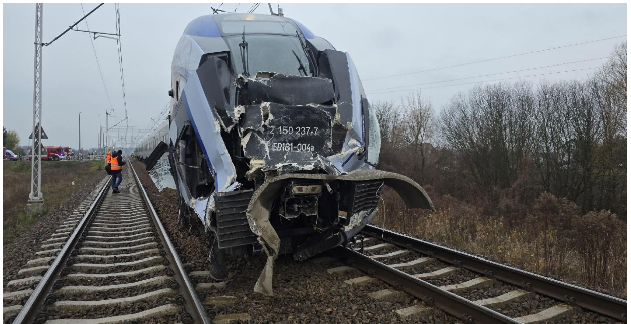
Photograph 2 – The consequences of the occurrence to the railway vehicle – damage to the cab and head of ED161- 004a (photo by the railway commission)
