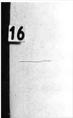
Transverse crack revealed by magnetic particle testing [EN 15313, §C.2.6 ]
