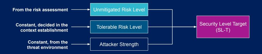
Security Level allocated at Zone level and on each Asset, based on 7 Foundational Requirements.
