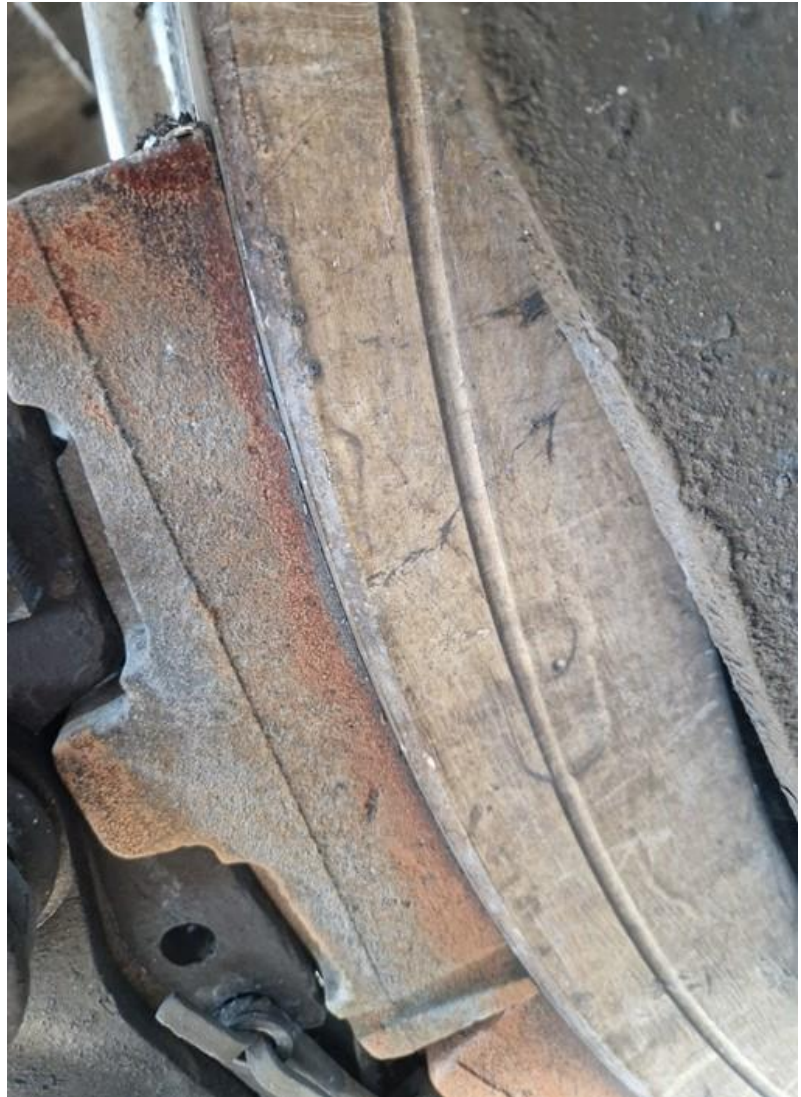
Fig. 4.19. Condition of the locomotive pad.
