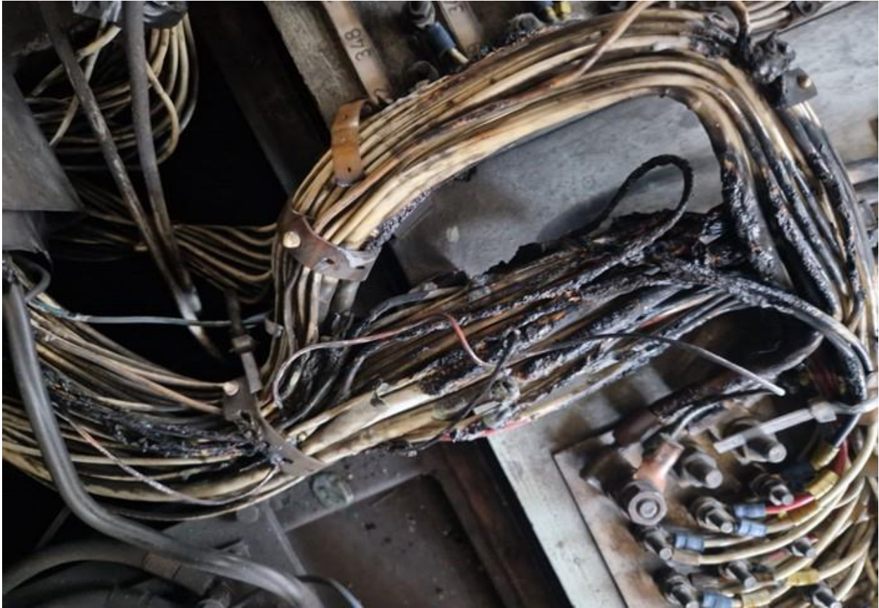
Fig. 4.16. Burnt cables on conductor 870.
