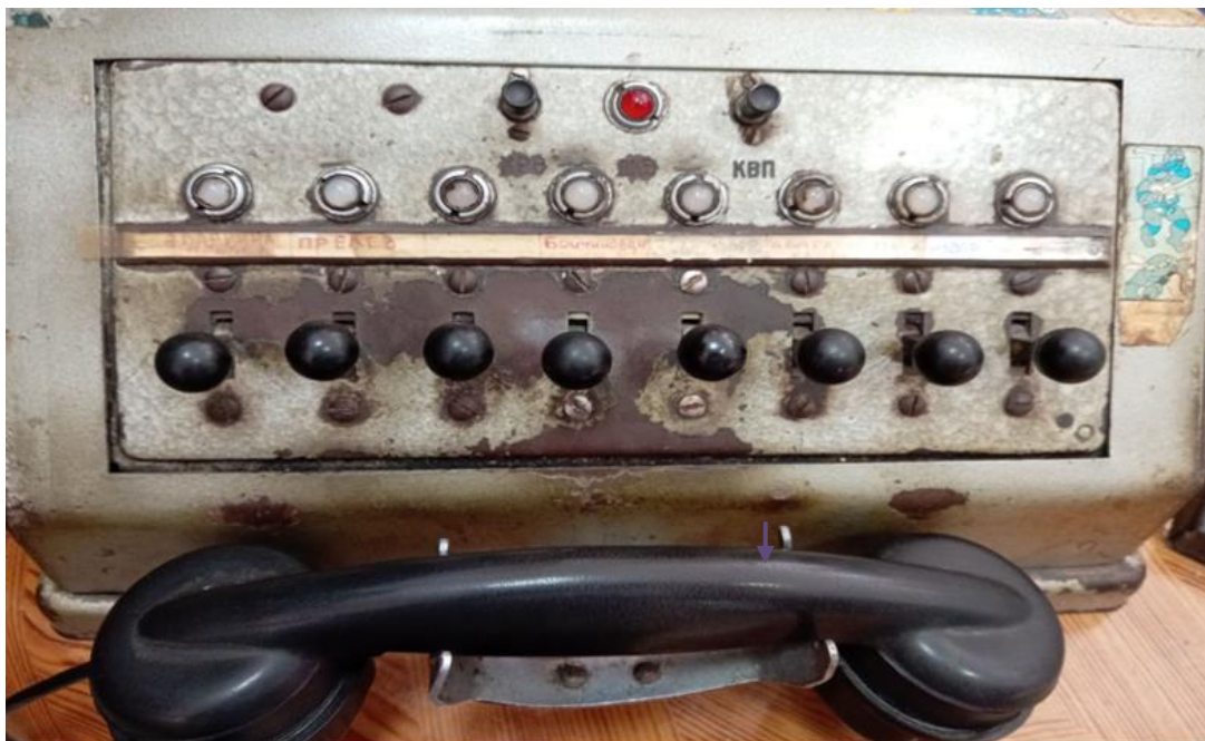
Fig. 3.12. Apparatus for direct interstation connection DCCM 8.
