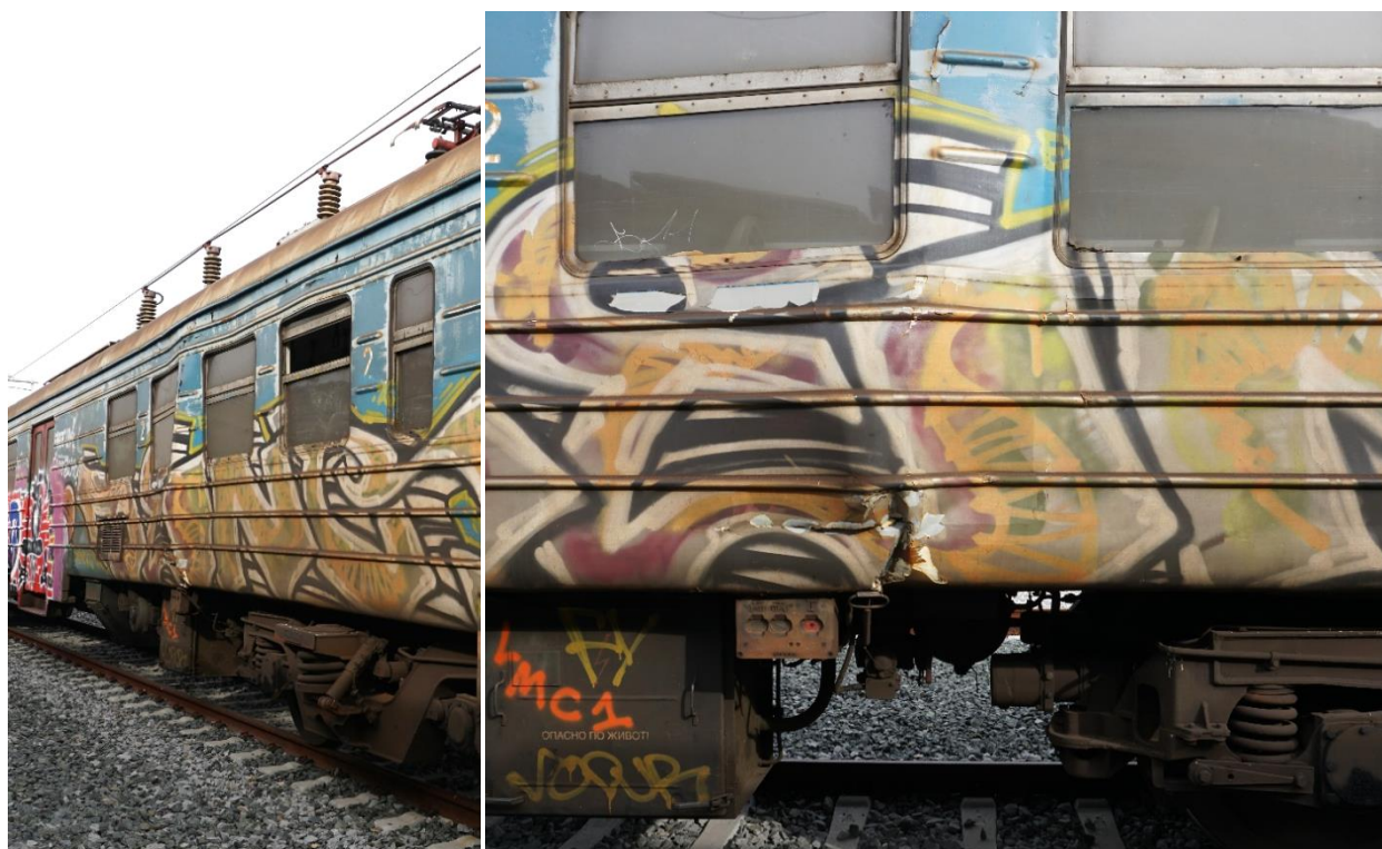
Figure 4.2.5.13: Appearance of the damage on the body of the trailer vehicle 416-013
