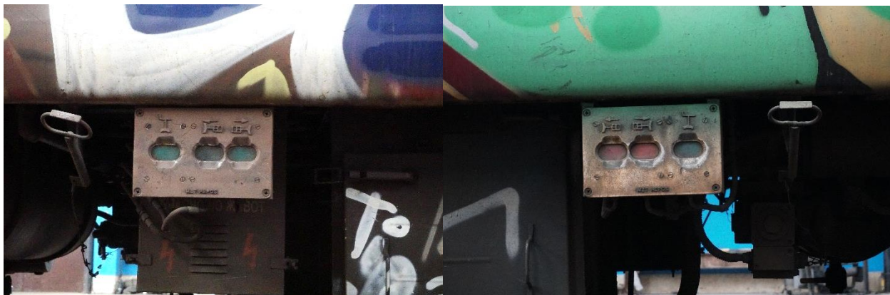
Figure 4.2.5.17: Appearance of the brake indicator on the trailer vehicle 416-013 (in the released position) and trailer vehicle 416-095 (in the locked position)
