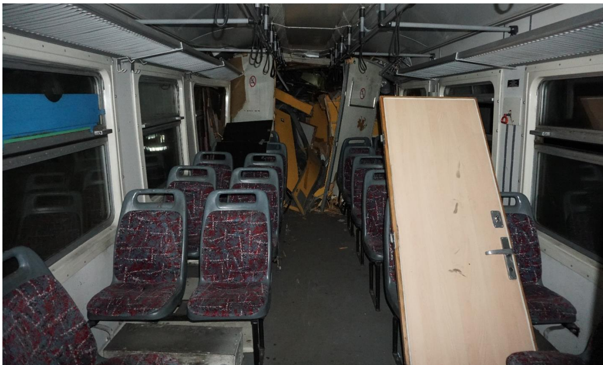
Figure 4.1.3: Appearance of deformations in the passenger compartment of the motor coach 412-005 of the train No. 7112 after the accident
