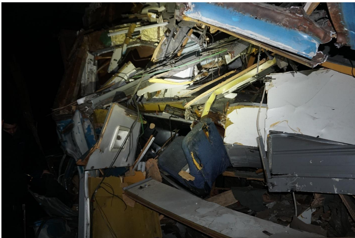
Figure 3.4.4.5: View of the driver's cab of the motor coach 412-005 of the train No. 7112 after the accident
