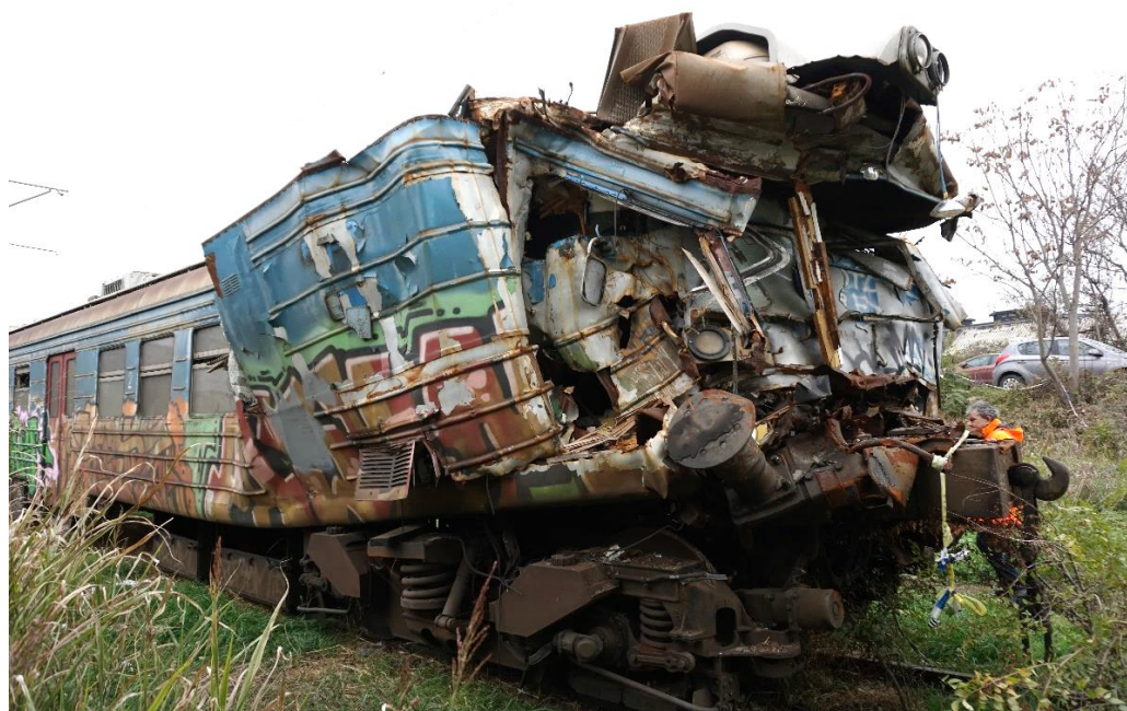
Figure 4.2.5.3: Appearance of damage to the front of the motor coach 412-005
