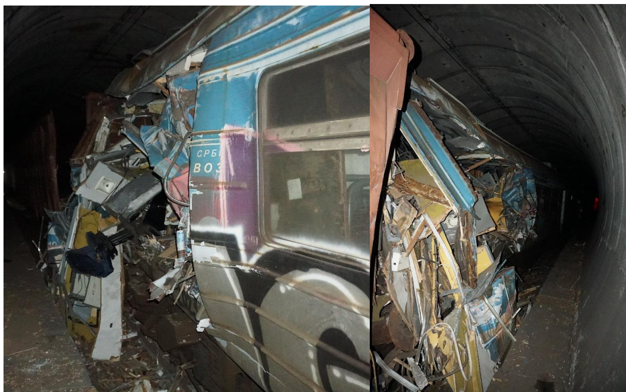
Figure 4.1.2: Appearance of damage to the front of the motor coach 412-005 of the train No. 7112 after the accident
