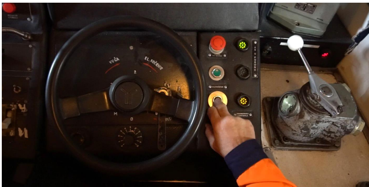
Figure 4.2.5.20: Appearance of the use of the "acknowledge" button and the indication of the time speed control
