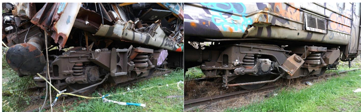
Figure 4.2.5.2: Appearance of damage to the bogies of of the motor coach 412-005
