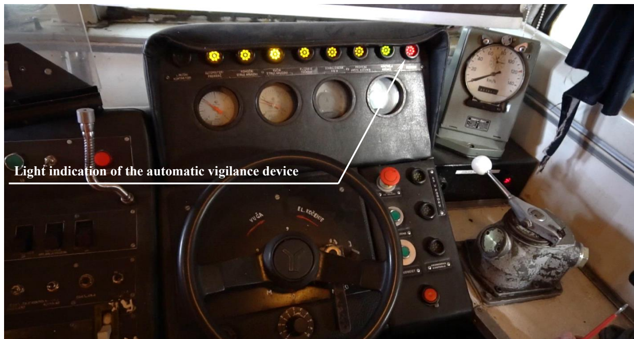
Figure 4.2.5.21: Appearance of the light indication of the automatic vigilance device
