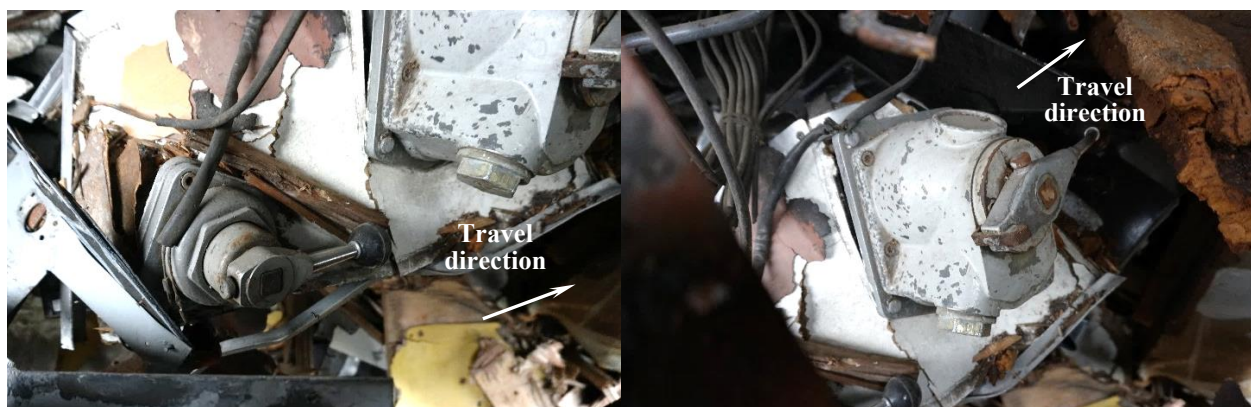
Figure 4.2.5.7: Appearance of the driver's automatic brake valve of the direct brake (left) and of the indirect brake (right) in the driver's cab of the motor coach 412-005
