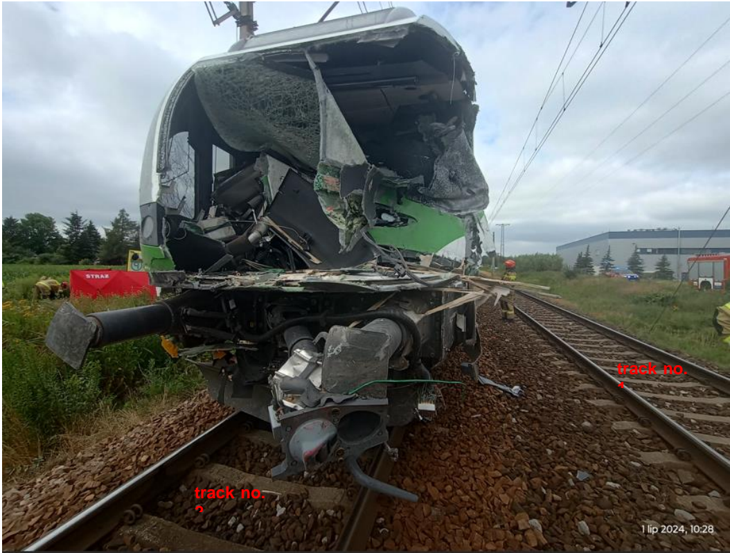
Photograph 6 - View of the damaged front wall of railway vehicle ER75-001 (source: KM)
