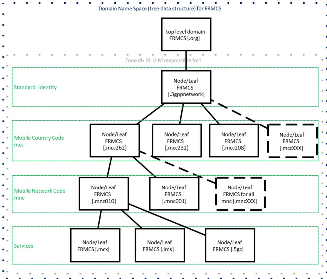
Figure 11-4: Domain Name Space for FRMCS (machine-type communication)
