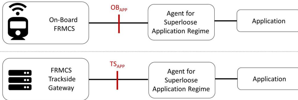
Figure 6-7 Superloose coupling mode
