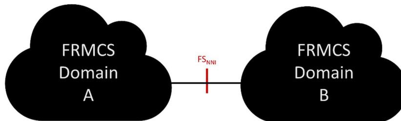
Figure 6-9 - FRMCS System: reference point between FRMCS Domains
