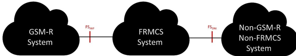
Figure 6-10 - FRMCS System: reference points towards external systems
