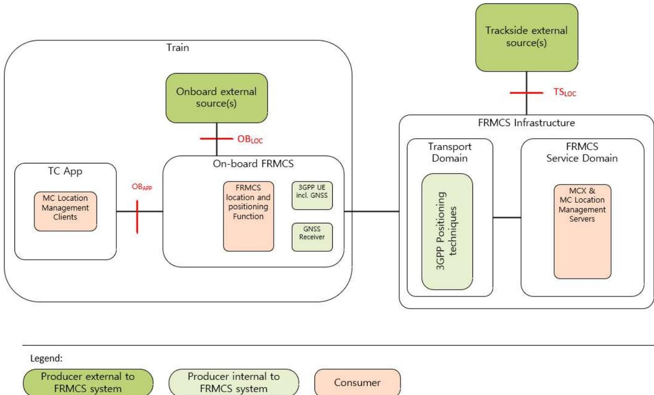
Figure 16-3 – Architecture of FRMCS Location and positioning system.
