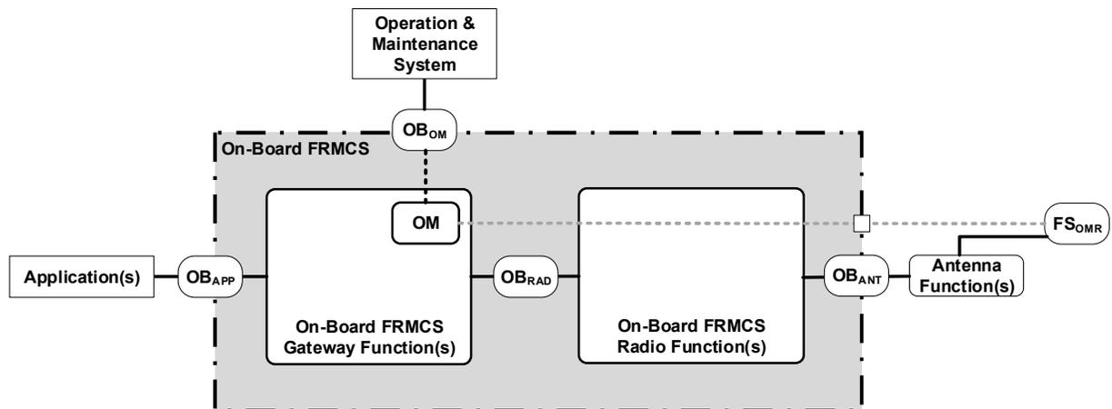
Figure 7-1: On-Board FRMCS architecture
