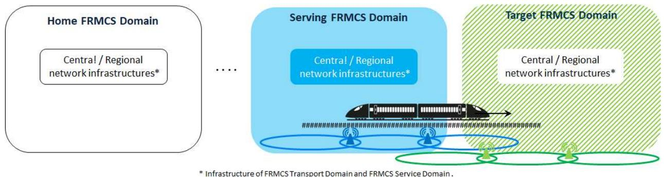
Figure 10-1. An example of an Inter-FRMCS-Domain transition
