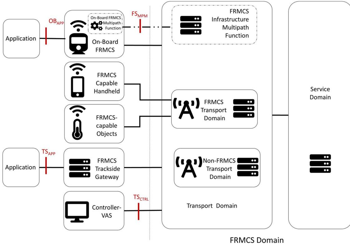
Figure 6-8 - System Reference Architecture
