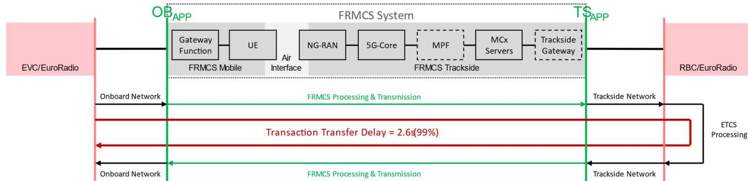
Figure A.3-1: E2E path for transaction transfer delay for ETCS
