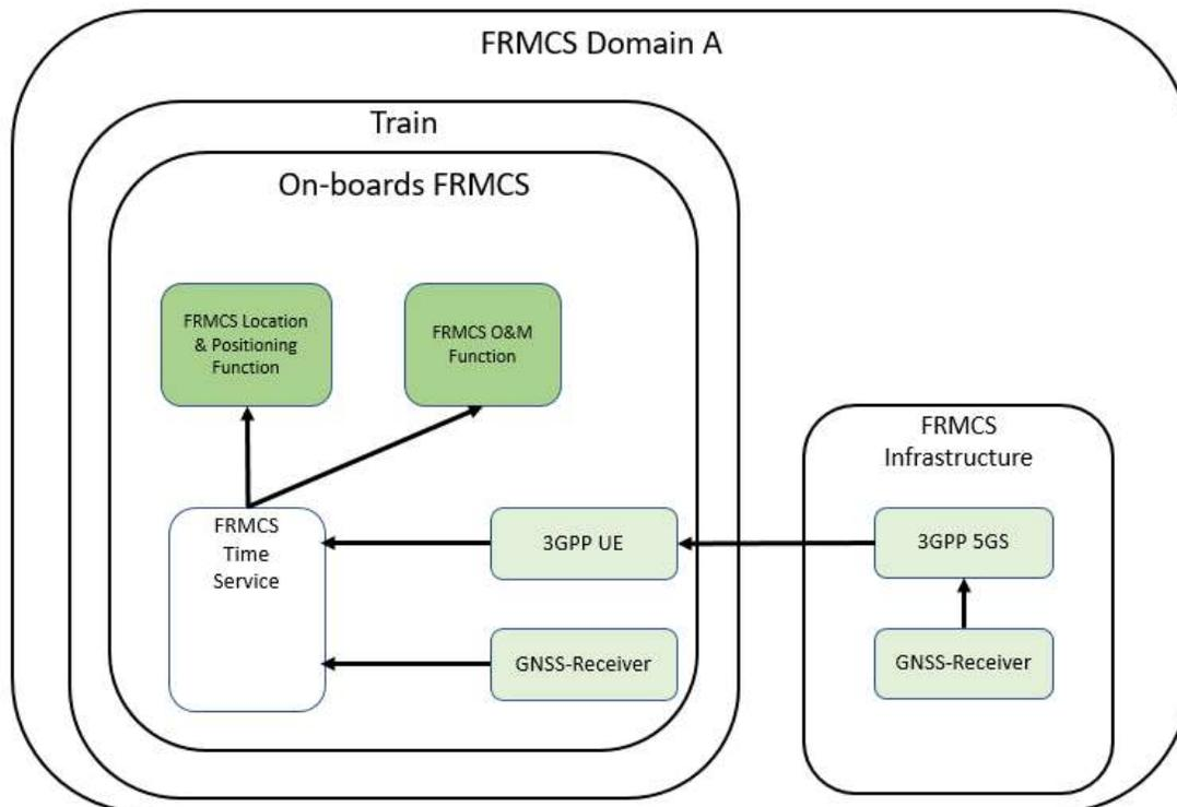
Figure 23-1 – Time Synchronization Flow
