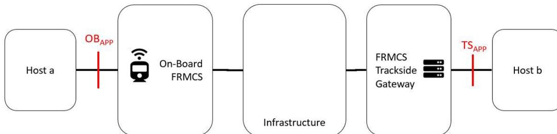
Figure 6-11: Host-to-Host (H2H) addressing principle (Loose-coupled example)
